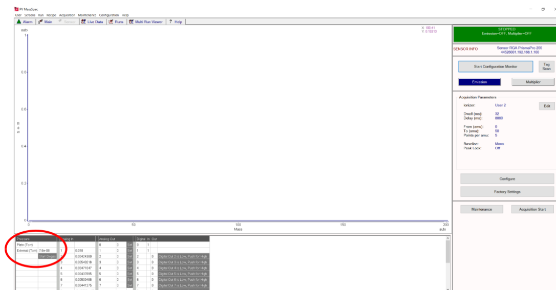
Figure 1: Set the pressure from external gauge.
