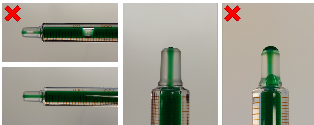
Figure 3: Utilizing a syringe with bubble free electrolyte and ensuring that only one liquid-gas interface is present within the syringe minimizes the risk of introducing bubbles into the EC-cell. The left images show a Hamilton syringe when bubbles are present (top) and when filled properly (bottom). Note that both bubbles in the tip and the body of the syringe are problematic. Furthermore, the syringe should have a small meniscus (middle image) upon insertion and injection into the cell as excess droplets (right image) may cause issues.
