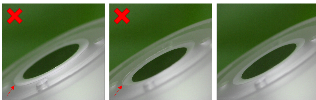
Figure 4: Correct mounting of disk and U-cup assembly in the EC-cell is important for minimizing the risk of bubbles as well as ensuring the overall performance of the EC-MS system. The surface of the disk and the U-cup should be completely flush with the cell (right). It is recommended to use either a magnifying glass or a microscope to verify that neither the disk nor U-cup are protruding (left) or indented (middle).
